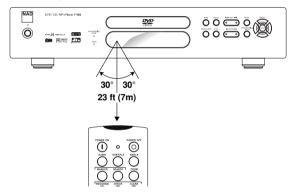
Distance: About 23 ft (7 m) from the front of the remote sensor Angle: About 30 degrees in each direction of the front of the remote sensor
